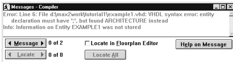
Figure B.24 The Message Processor window displaying an error in VHDL code.
