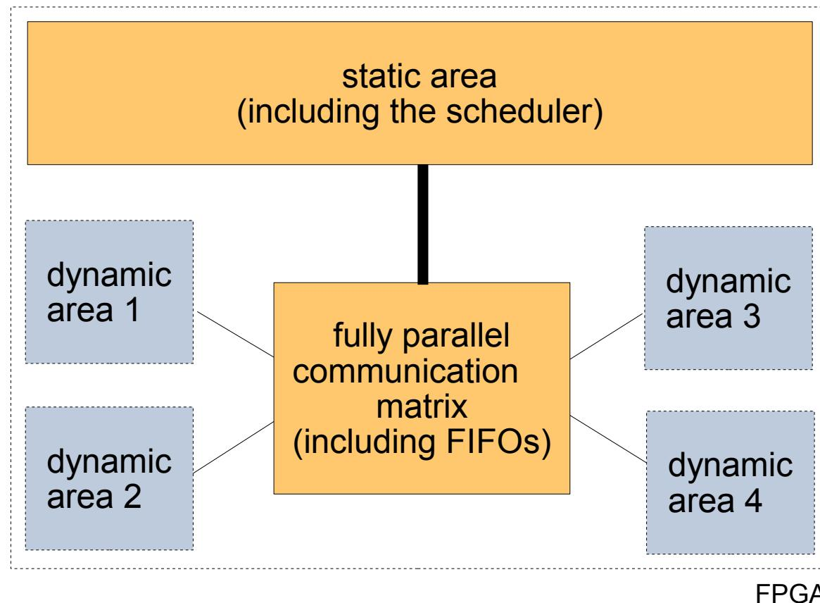
*Modules are loaded into the dynamic areas **on demand**. The communication matrix stores the data for every module in a FIFO. Since there is a farm of FIFOs the communication between several modules is fully parallel.*
