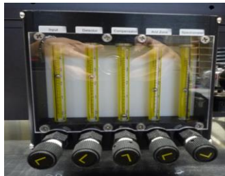
2.4, 2.4, 0 , 1.4, 1.4 Note: The flow rates are a little higher than what the manual said because there was a problem with the stability of CO 2 /H 2 O concentrations before (by Robert).
