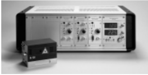
Rubidium Saturation Spectroscopy Teaching System
