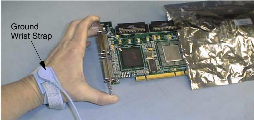
**Figure 2-7. Remove the controller from the Anti-static Bag**
